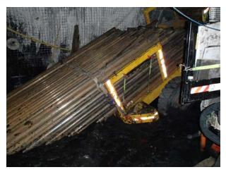
Where the process of using a trailer or other load-carrying device can result in varying loads, controls should be in place to manage the risk of unbalanced, uneven and shifting loads.
