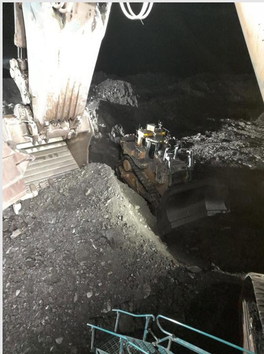
Dozer operators must maintain a safe distance when operating in close proximity to excavators (must remain outside of the excavator swing radius). Machine operators should not rely on experience or previous movements of other operators as a substitute for positive communications. Refer to [Safety Bulletin 18-06 Lack of positive communications](#) which addressed similar incidents.
