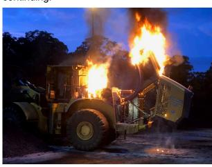
Any machines fitted with burn type diesel particulate treatment should have the risk of this process addressed in the fire risk assessment for the machine.
