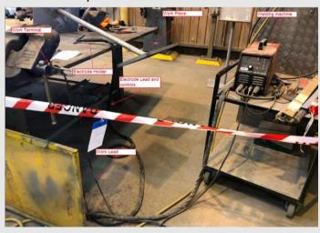
All welding equipment should be inspected before use and should be properly maintained.
