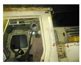
Open-ended, low-hanging pipes are an easily identifiable hazard and present an unacceptable risk to vehicle operators. Mine operators should have controls in place to eliminate/mitigate risks that can arise from such a hazard, such as hanging the pipes at a height where they do not align with the travel path of a vehicle.
