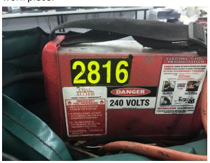
People involved with welding activities should remain insulated from the welding job. Welding gloves are not electrical insulators and if they are damp, they can enhance the effect of an electric shock.
