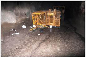
Mine operators must ensure that locking pins are in place on mobile plant used for work boxes. The locking pins should be used to give a positive/secure attachment. Mine workers involved in the task must verify that all locking pins are correctly engaged prior to use.
