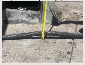
From the primary investigation it was identified that the rope may have been run over by a vehicle with rubber tyres. Mines operating winders should have exclusion zones clearly defined. Workers must report damage to plant and equipment when it occurs.
