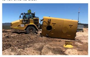
Mines that are operating articulated vehicles, particularly water carts, should review operating parameters (include slope and cross grades). Work areas should be assessed to determine if articulated vehicles are the correct plant for the task.
