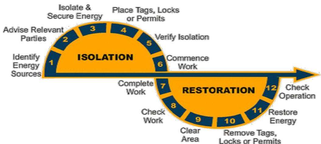
Fluid power systems are often powered by energy sources such as electricity or diesel engines. These power sources must be part of the isolation consideration. Isolate and secure all energy sources.
