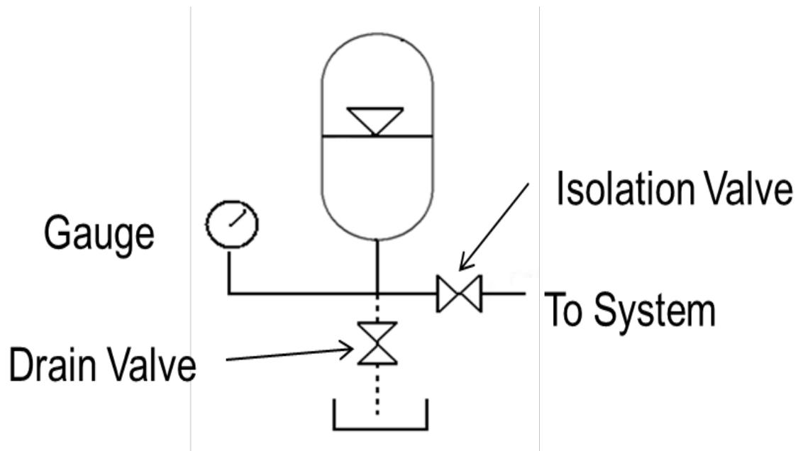
**NEVER** try to disassemble an accumulator without **FIRST** releasing the pre-charge gas.
