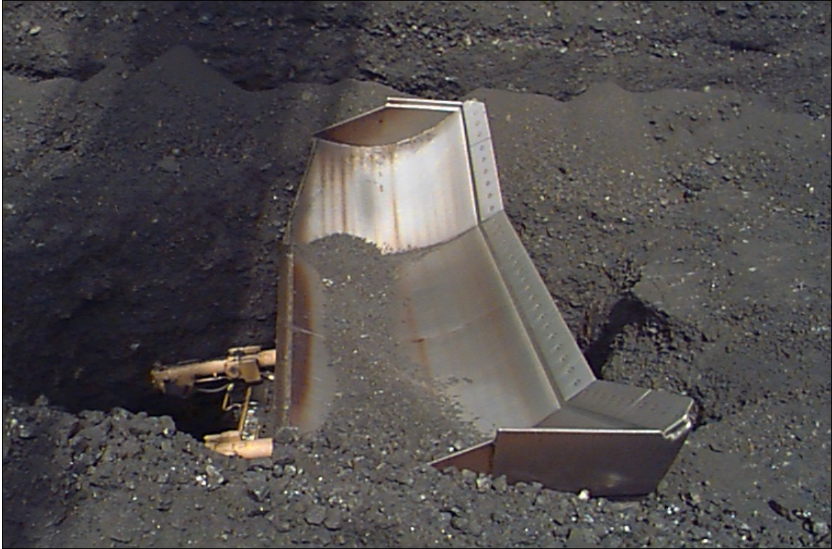
Figure 1. A stockpile dozer has fallen backwards when a bridged draw down point suddenly collapsed.
