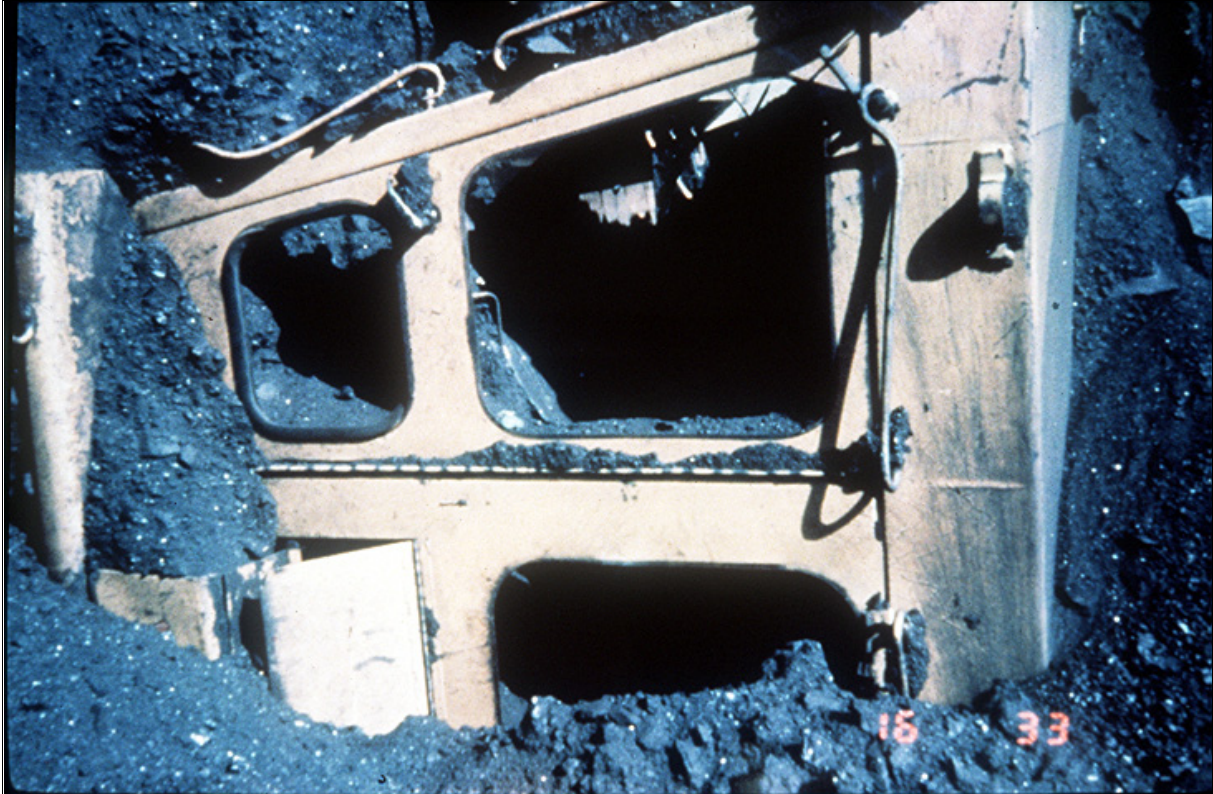
Figure 5. Windows in the driver's cabin of this stockpile dozer have collapsed and the cab filled with coal after the dozer fell into the draw down point.
