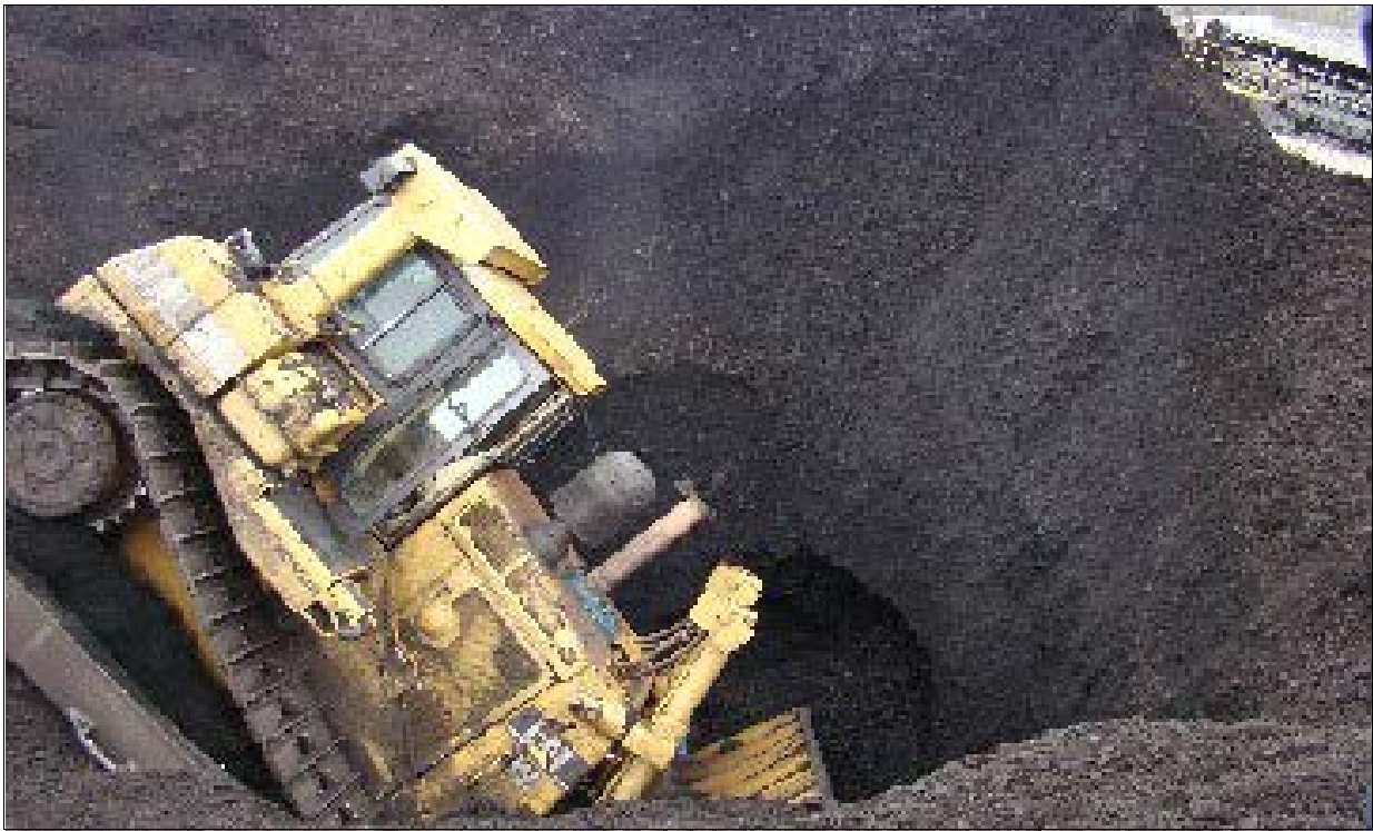
Figure 2. The dozer driver has driven into the draw down point.
