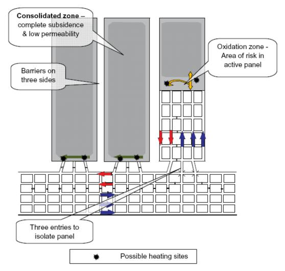
Figure 3 shows an arrangement where panels are not isolated by barriers and instead have reduced to manageable size by a line of stoppings. Areas of risk where heatings may occur in the goaf are shown. This assumes no interconnectivity from the surface, boreholes, or workings in another seam.
