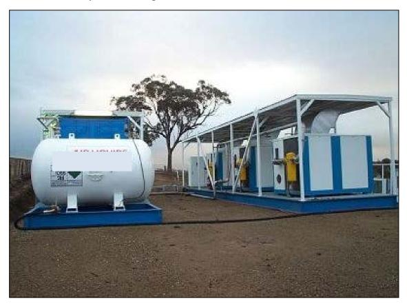
Figure 31: Membrane Separation Generator technology
