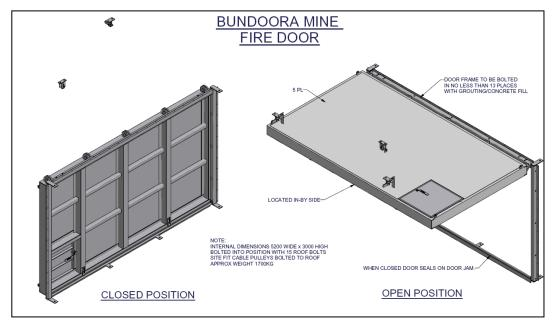
Figure 40: Remote door arrangement in an underground mine
