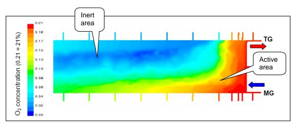
Figure 7: CFD Model of Goaf Atmosphere
