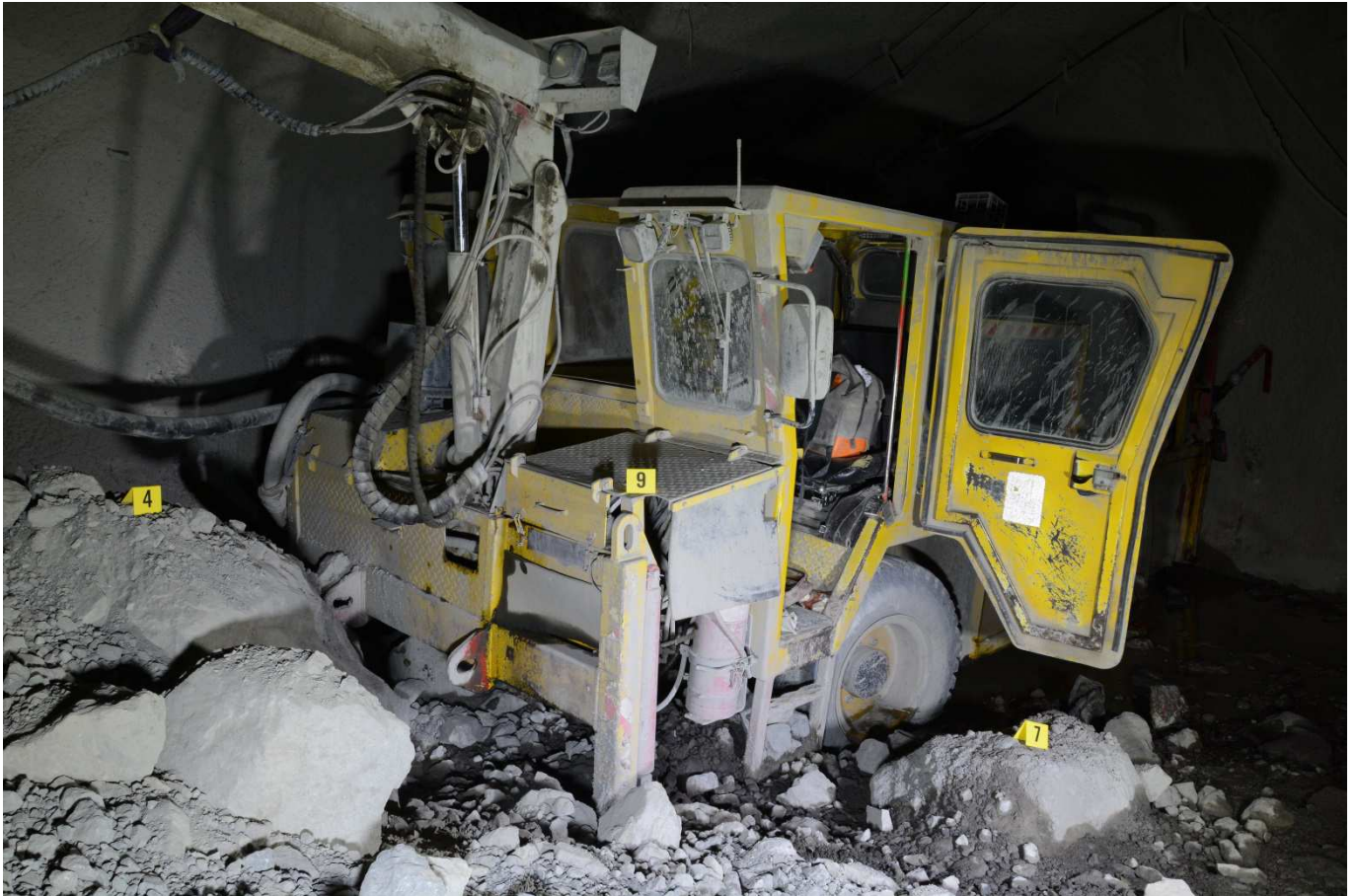
Figure 14 Photograph of a large rock that was contacting the front of the water cannon after excavating around it.
