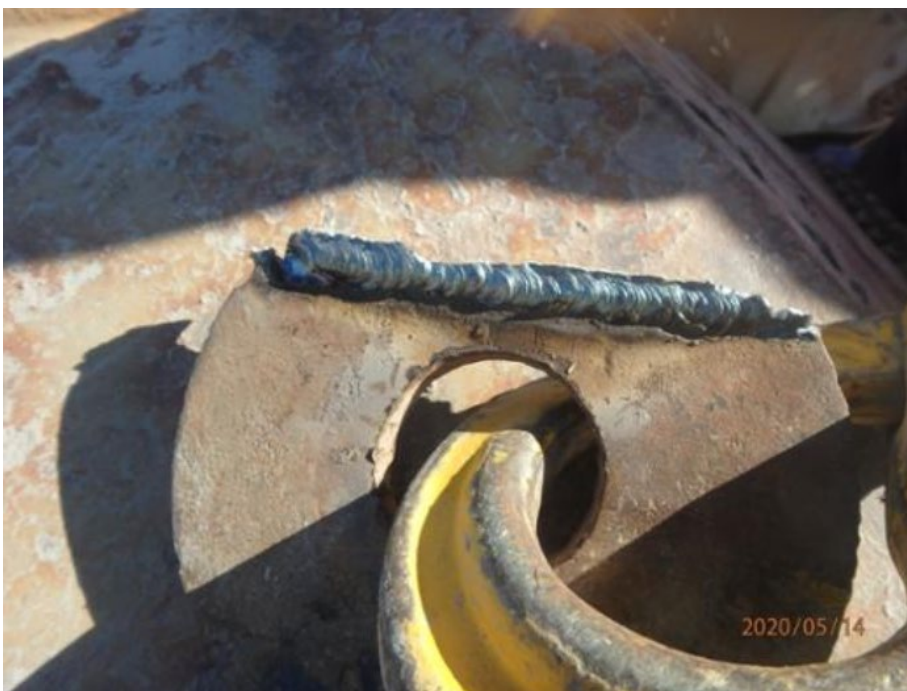
Figure 4 Failed lifting lug attached to lifting hook
