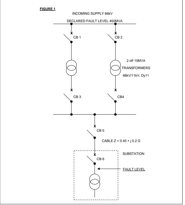
Using a base of ten (10) MVA, determine the fault level on the load side of circuit breaker - 6, (CB 6) when:
