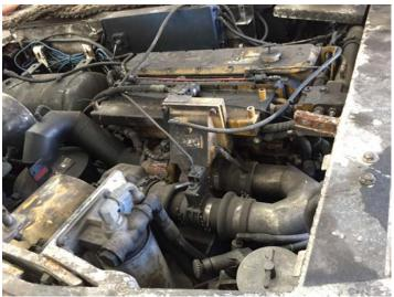
A scene preservation notice was issued and the machine was seized. It was removed off-site for inspection by an independent assessor. Visual inspections indicated a damaged oil supply pipe. This may have been a result of the engine failure or it may have been a precursor to the engine block failure. The causal investigation will seek to identify the exact causes of the failure.
