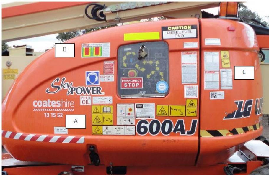
Fig 2: OEM signage provided adjacent to Ground Controls including Emergency Stop, refer operator manual, electrical hazard, tip over hazard, excessive side force hazard, crushing hazard and Emergency Control operation.
