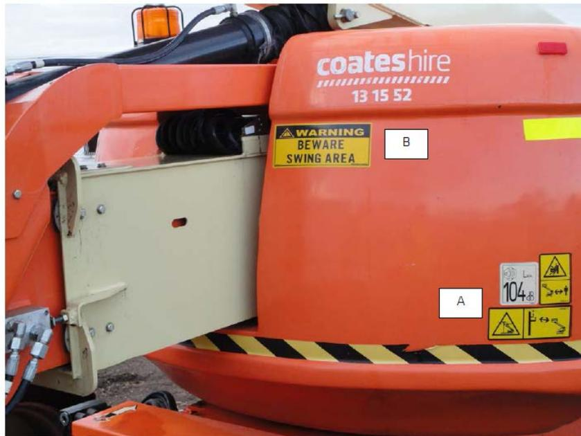
Fig 4: OEM signage provided on rear of EWP including crushing hazard (A) and Swing Area (B).
