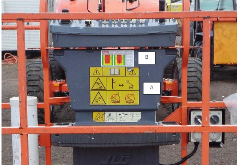
Fig 1: OEM signage (A) provided in platform including refer operator manual, electrical hazard, tip over hazard and excessive side force hazard.
