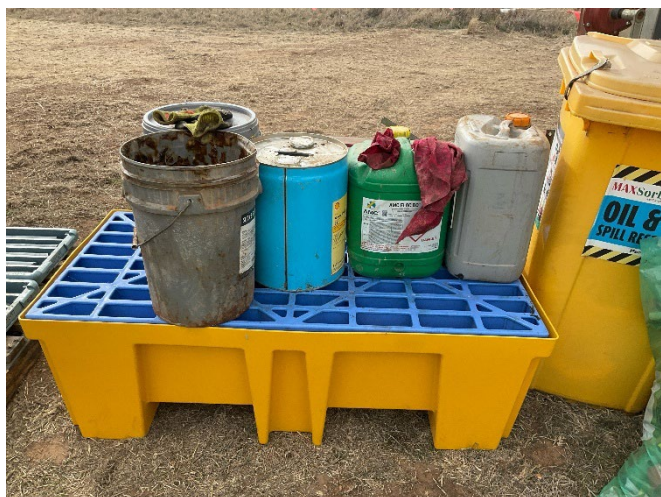
Figure 7: Use of aboveground sumps for diamond drilling
