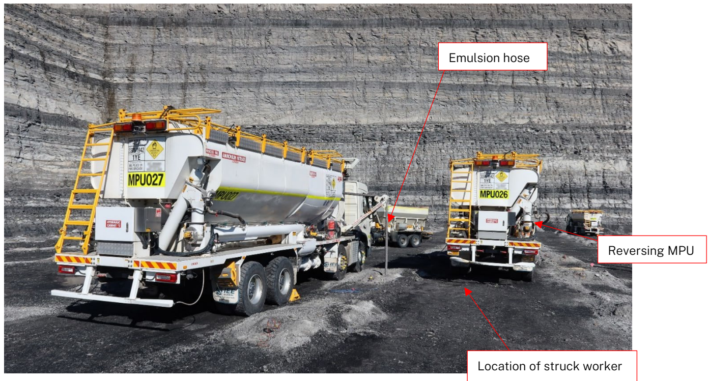
Figure 1 The 2 mobile processing units following the incident
