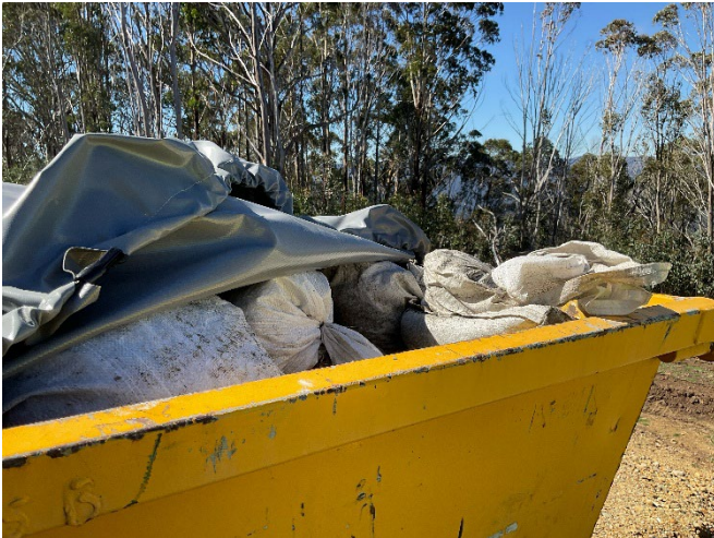
Figure 5: Dried drill cuttings in covered waste bin
