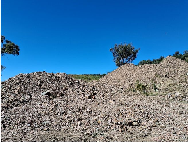
Figure 3: Topsoils stockpiled near entrance to the open pit
