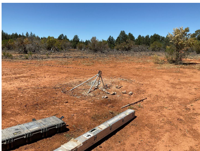
Figure 1: Downhole EM survey in progress on hole NMD115
