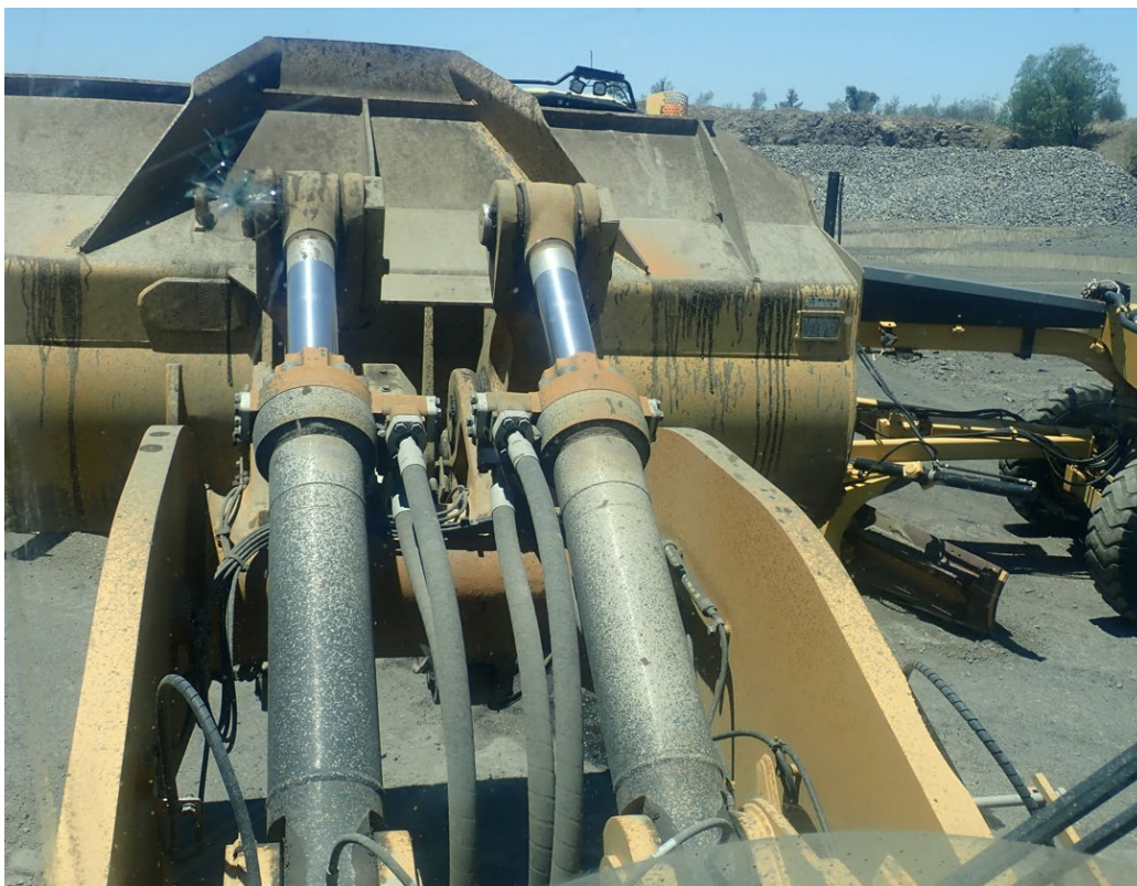
Figure 2 – Incident re-enactment photo showing obstructed view of the loader operator
