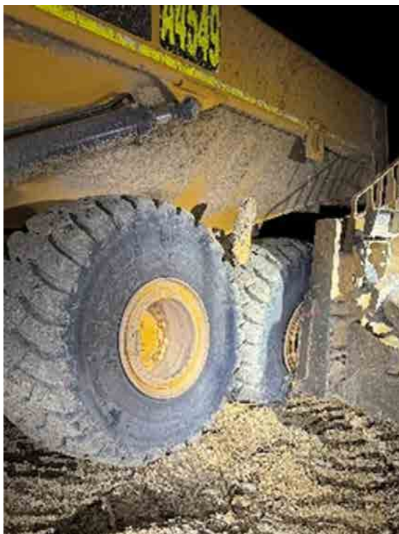
Picture 6. Scene of collision showing damaged tyre.
