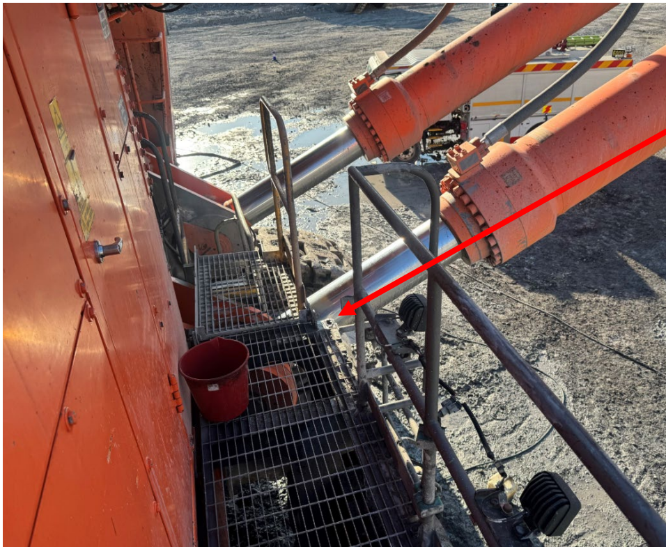
Figure 4: Location of failed handrail section on the excavator
