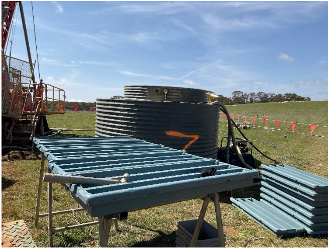
Figure 6: Above ground sumps for water management during diamond drilling
