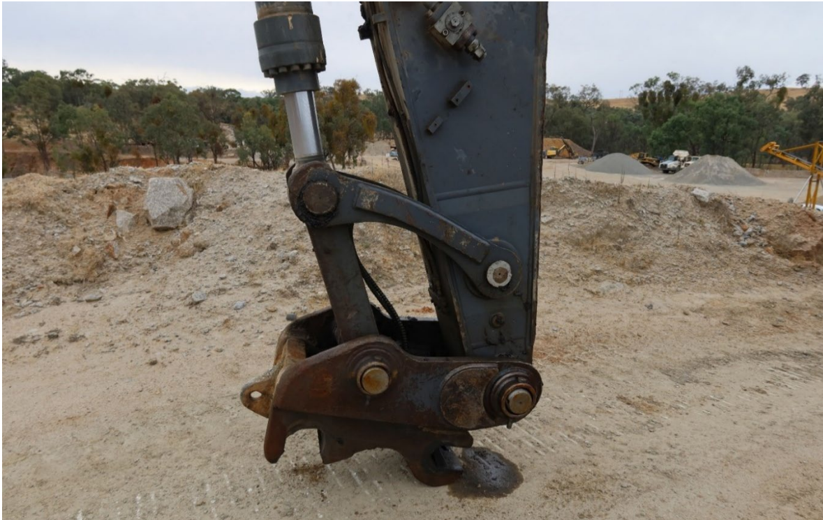
Figure 3: The quick hitch device on the excavator arm
