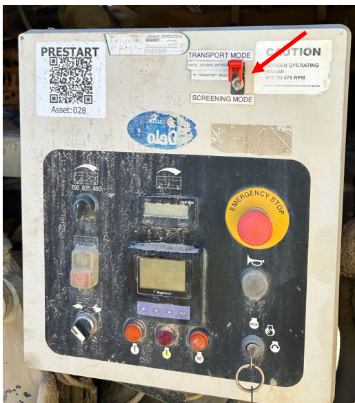
Figure 4: Toggle switch used to control operating mode, was changed over at the time of inspection
