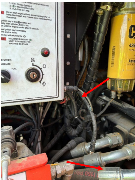
Figure 2: Travel plug inserted instead of operational plug. No labels identifying plugs.
