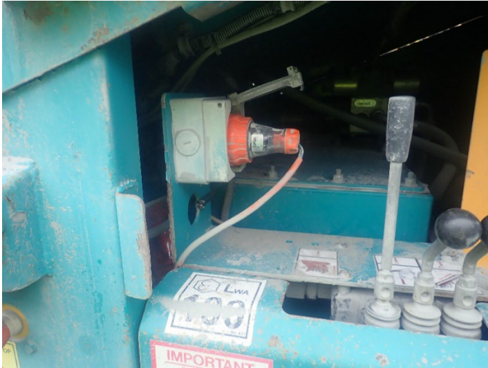
Figure 3: Travel plug inserted and no label to identify plug operation
