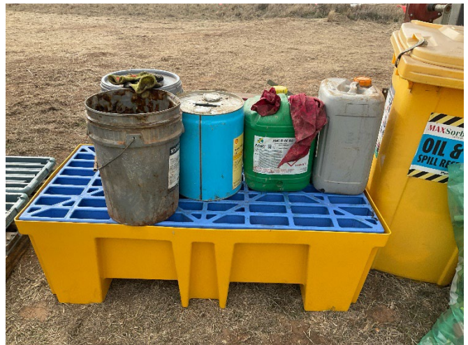
Figure 4: Fuels and oils on bunded spill pallet with stocked spill kit available
