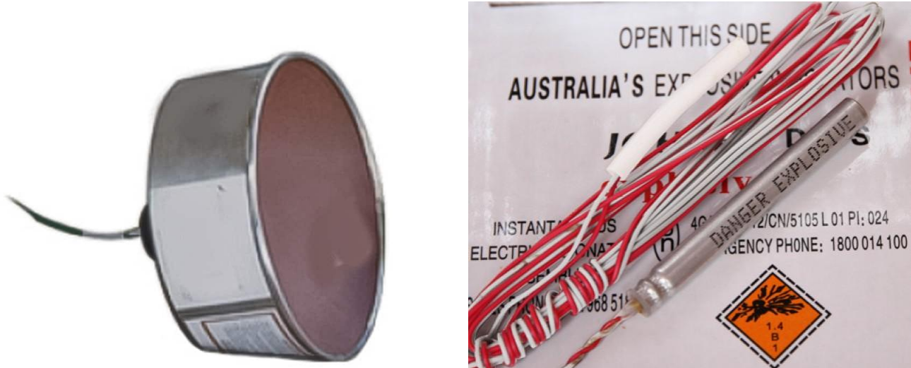
Figure 2: Photo of a ballistic disc (left) and an electric instantaneous detonator
