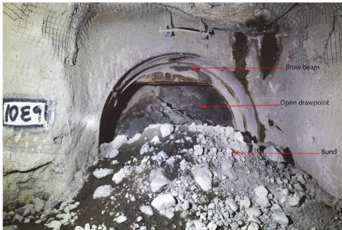
Figure 1: Photo of a drawpoint (not related to incident)
