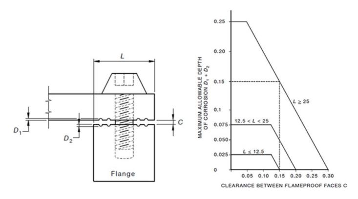
After inspecting indentations on the flame path, you find D1 measures 0.08mm and D2 measures 0.07mm and a 0.1mm feeler gauge will not fit into the enclosure gap C. From the certification drawings the flame path length is 28 mm.
