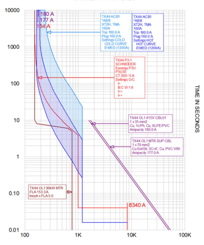
TX44 Outlet 1 Overcurrent.tcc Ref. Voltage: 415V Current in Amps x 1
