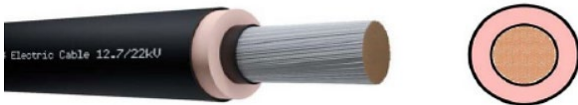
Figure 2: Example illustration of a single core 120 mm 2 ethylene propylene rubber (EPR) insulated panel wire 12.7/22kV
