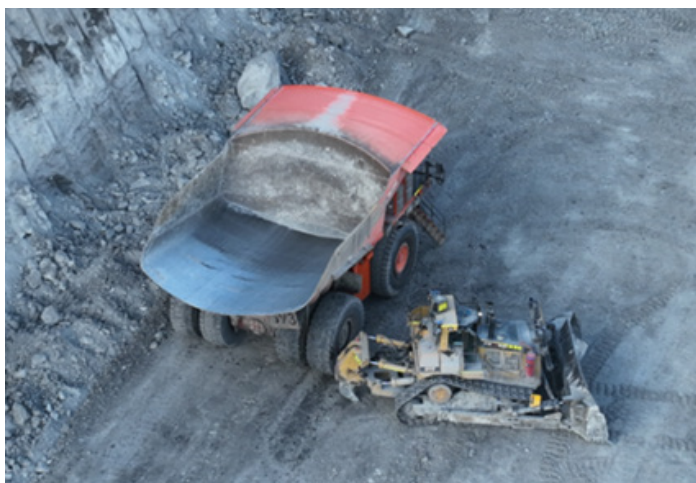
Picture 10. Contact between dozer and dump truck
