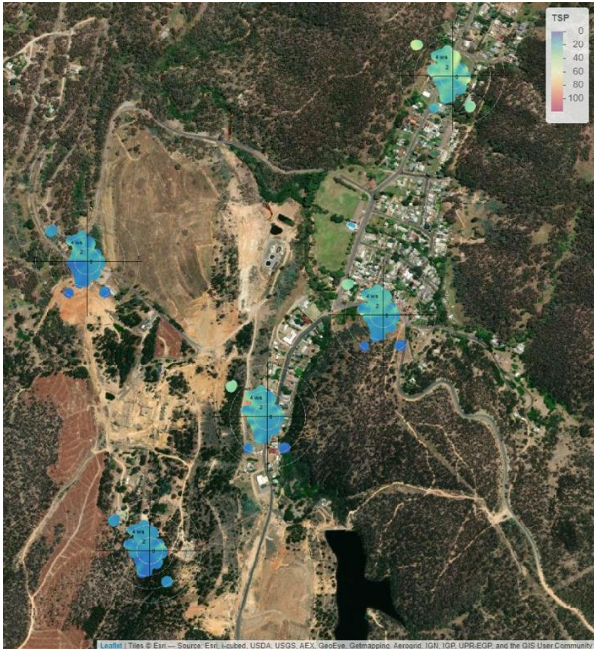
Figure 7-1: Polar map plots showing 24-hour TSP concentration ( \mu\text{g}/\text{m}^3 ) and 24-hour average wind speed and direction at each monitoring location, from 22 June 2021
