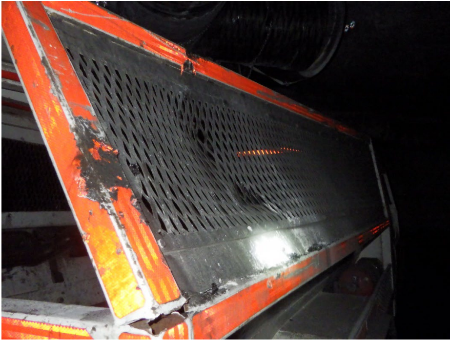
Figure 5: Damage to personnel transport caused by collision with shuttle car
