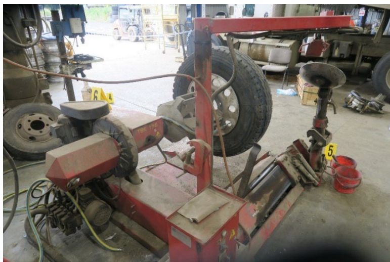
Figure 3: Compressed air line hose and high-flow coupling fitted to the tyre and wheel assembly
