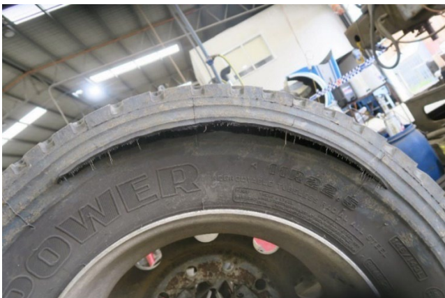
Figure 4: Front view of tyre showing side wall failure
