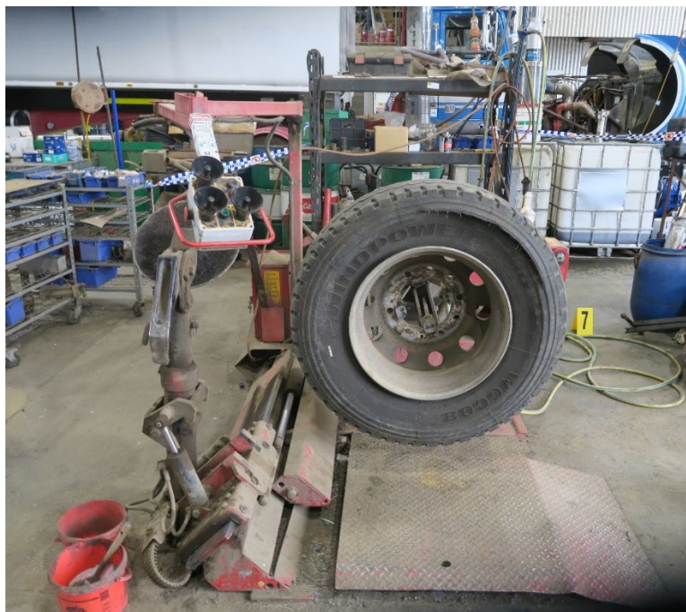
Figure 2: Rear view of tyre and wheel assembly fitted to tyre-fitting machine after the incident
