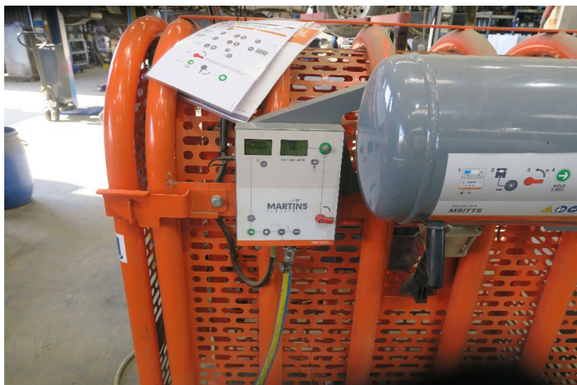
Figure 7: Tyre inflation cage used at Clovass Quarry post incident
