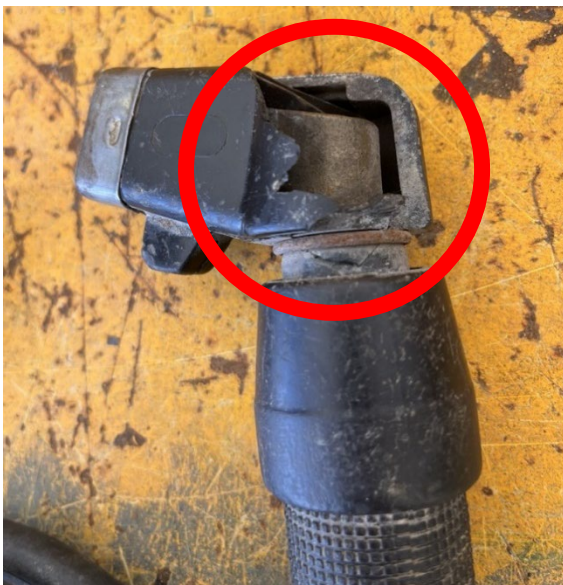
Figures 8 & 9: Damage to welding handpiece, and battery portable welder
