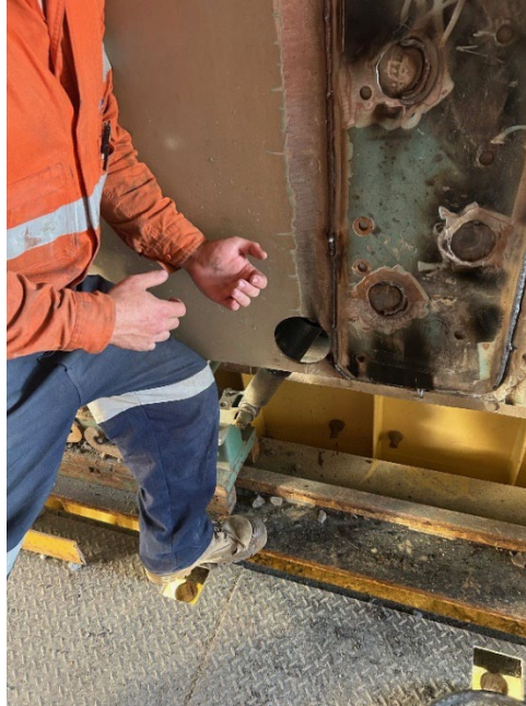
Figures 6 & 7: Earth clamp location on screen, and reenactment of boilermaker position while welding
