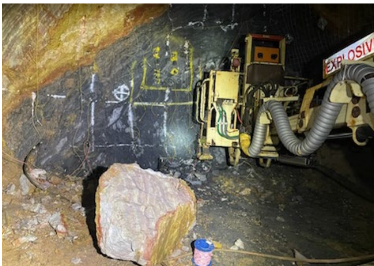
Figure 1: The 2-3 tonne rock that fell from the face
