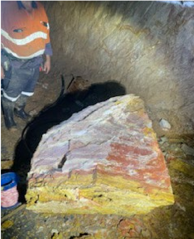
Figure 2: Worker standing next to the fallen rock showing the scale of the rock that hit the worker
