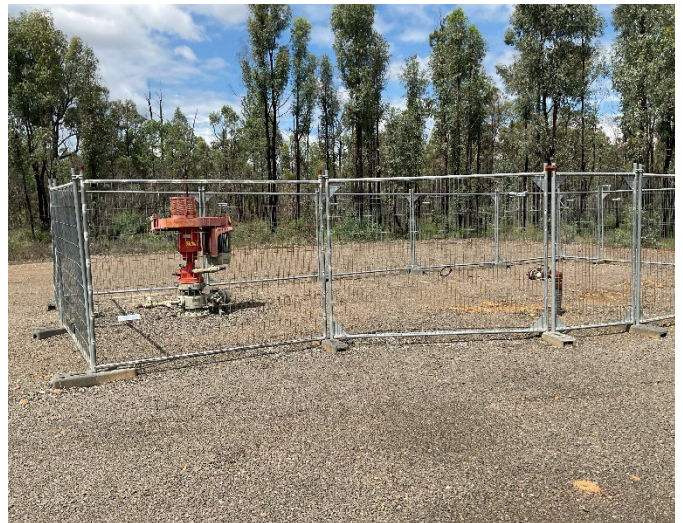
Figure 13: Handles locked or removed at Wilga Park 1
