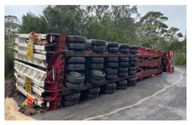
Operators must identify the risk of loads shifting due to an imbalance, especially when there is steel-on-steel contact.
