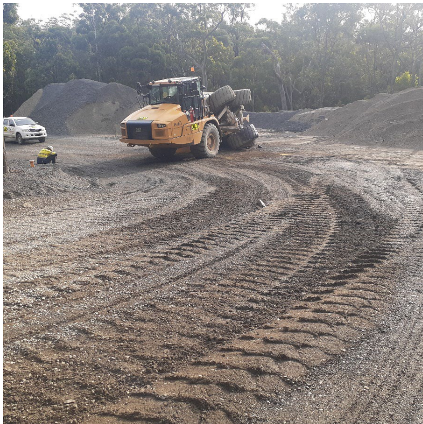
Figure 3: Road conditions contribute to rollover of rear tub
