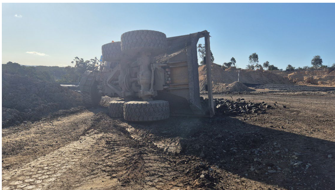
Figure 3: Road conditions contribute to rollover of rear tub
