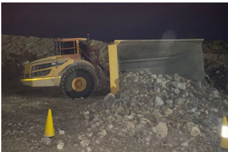
Figure 1: Reversing into windrow resulting in tub section rolling and discharging load
