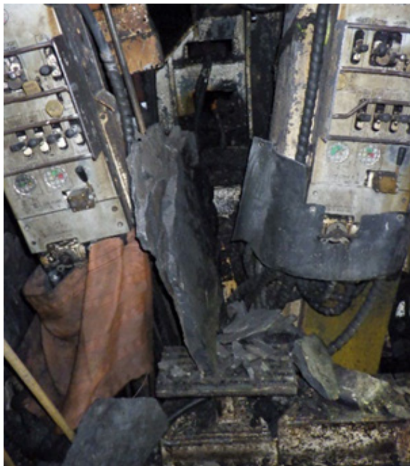
Picture 2. Slab resting on continuous miner platform after incident
