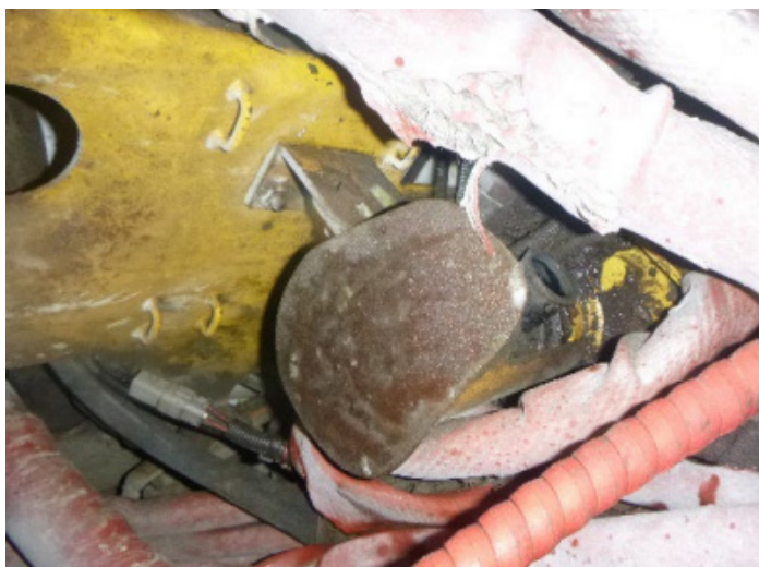
Picture 19. Loose breather hose on haul truck
