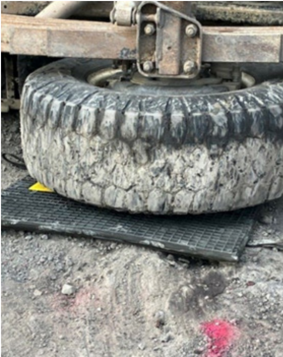
Picture 14. Worn tyre on rolled light vehicle
