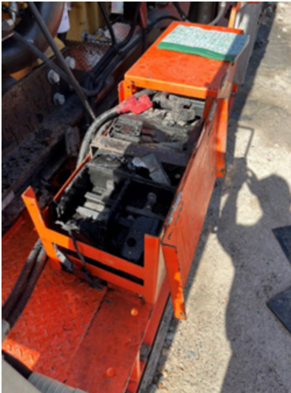
Picture 17. Battery enclosure minus unsecured lid
