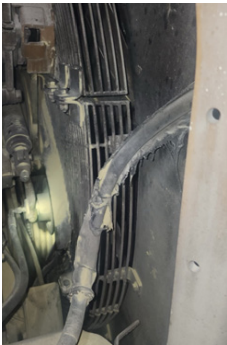
Picture 16. Hose damage at rear of dozer
