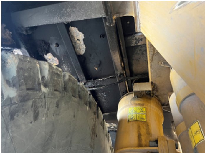
Picture 18. Fire location underneath right-hand fender
