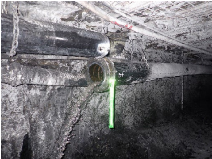
Picture 6. Fractured poly pipe
