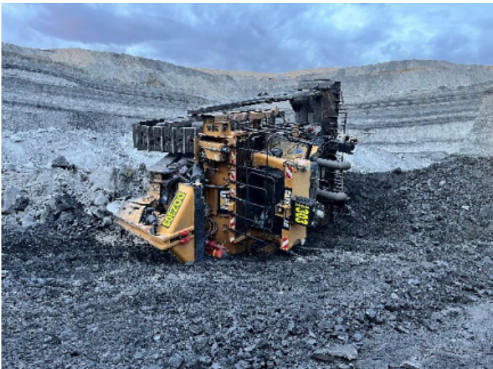
Picture 7. Tipped dozer at dig area
