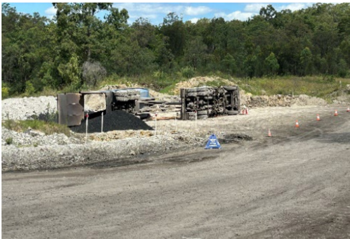
Picture 9. Tipped mover and trailer
