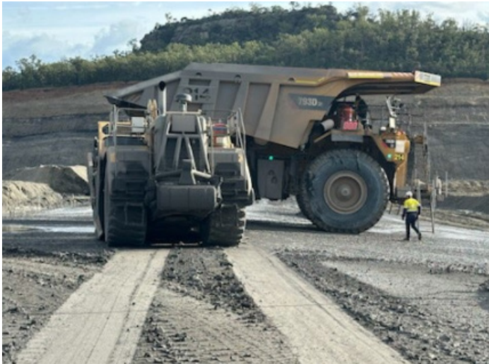
Picture 12. Scraper and haul truck with visible slide marks
