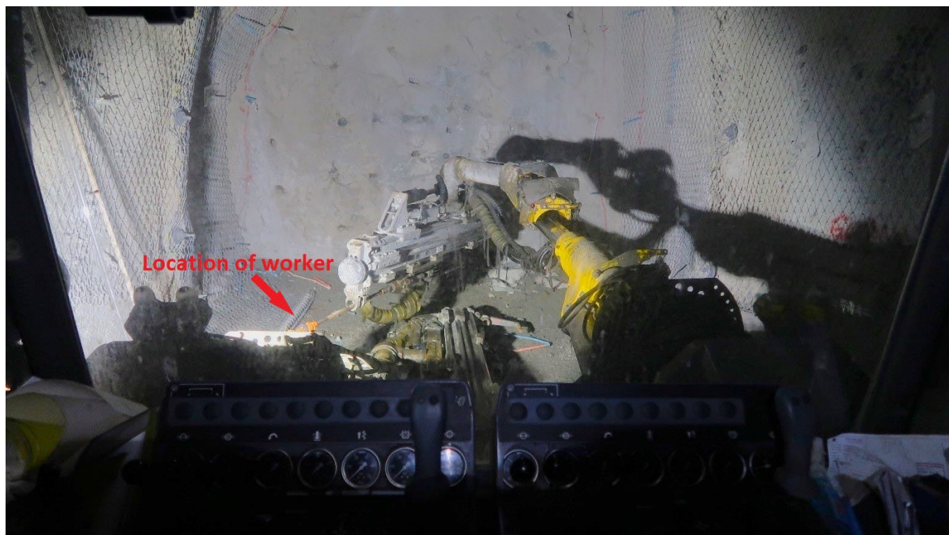
Figure 2: Incident scene viewed from the jumbo cabin with approximate location of offsider at the time of the incident, and a piece of his work shirt (predominantly orange in colour) entangled in the drill steel
