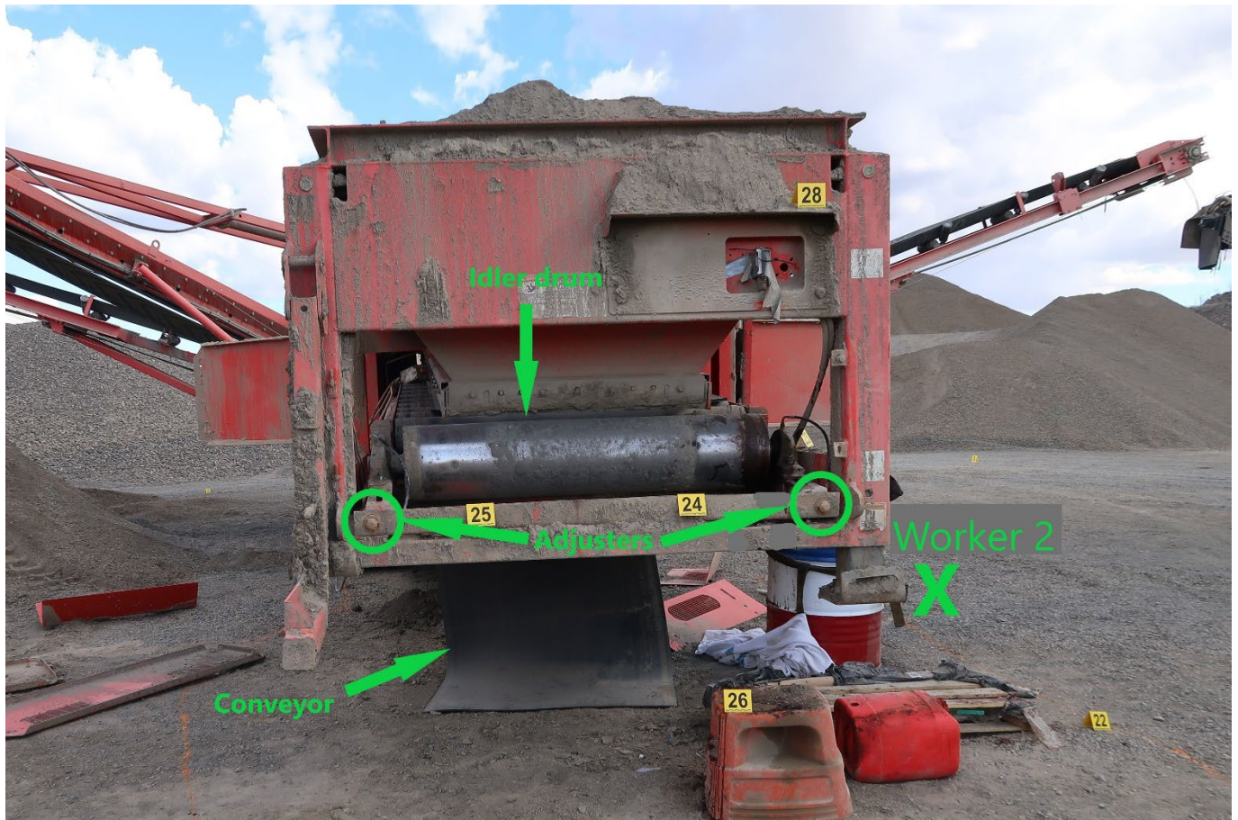
Figure 2: Depicts the rear view of mobile screen with relevant parts identified and the approximate location of worker 2 at the time of the incident labelled (Note: the conveyor belt was cut during rescue efforts)
