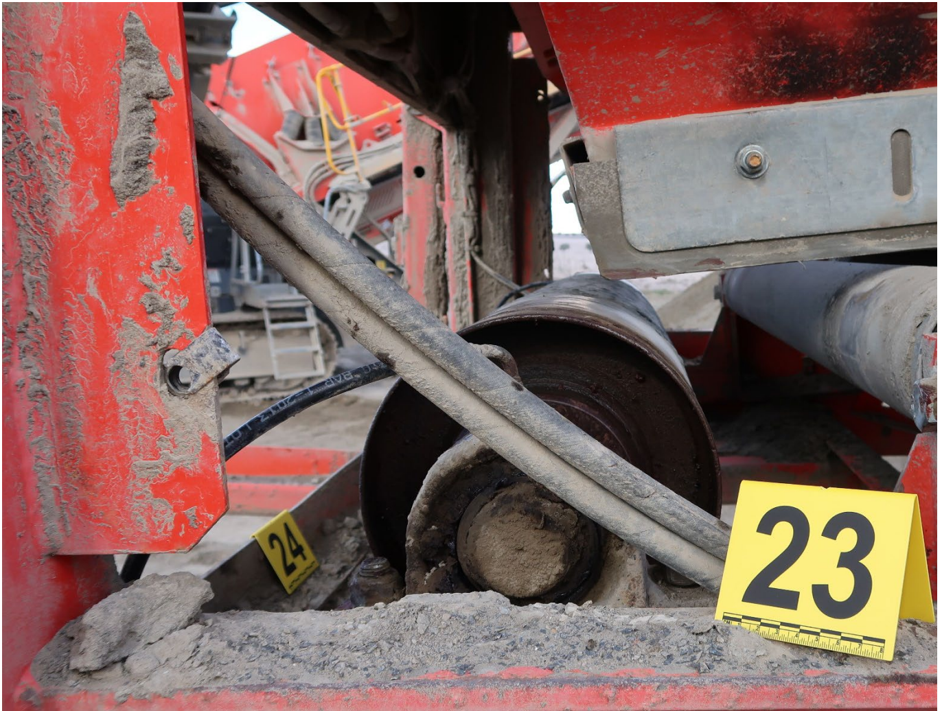
Figure 3: Depicts a close-up view of the tail drum taken through right-hand guard door where the injured worker was positioned
