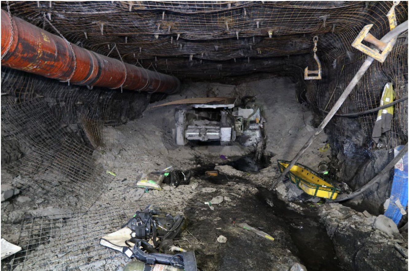
Figure 1: The continuous miner partially buried in rock material in Razorback Mains B heading 11-12 cut-through
