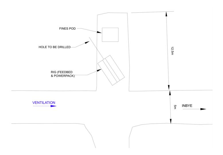
C) Referring to the stub setup sketched above, how would **the deputy** control the risks associated with the drillers operating on the travel road for the inbye development panel – identify at least 3 (three) controls. **(1 mark)**
