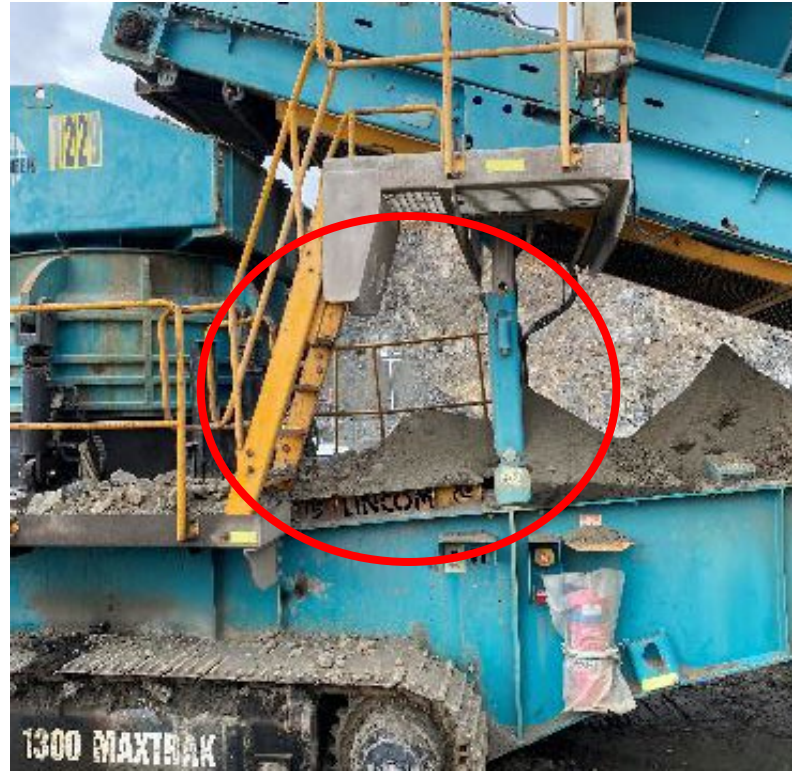
Exposed fall area & build up
