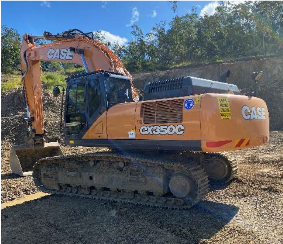
No fall protection around engine bay
