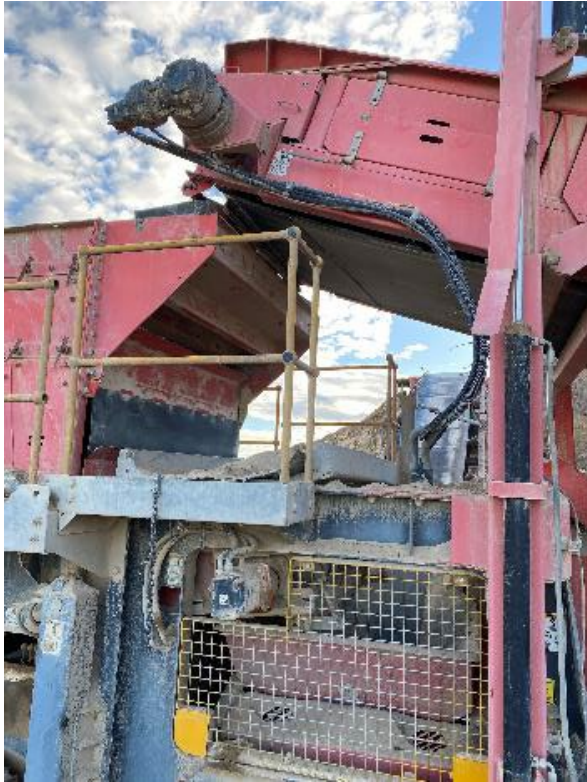
Missing handrail & no head clearance to moving belt
