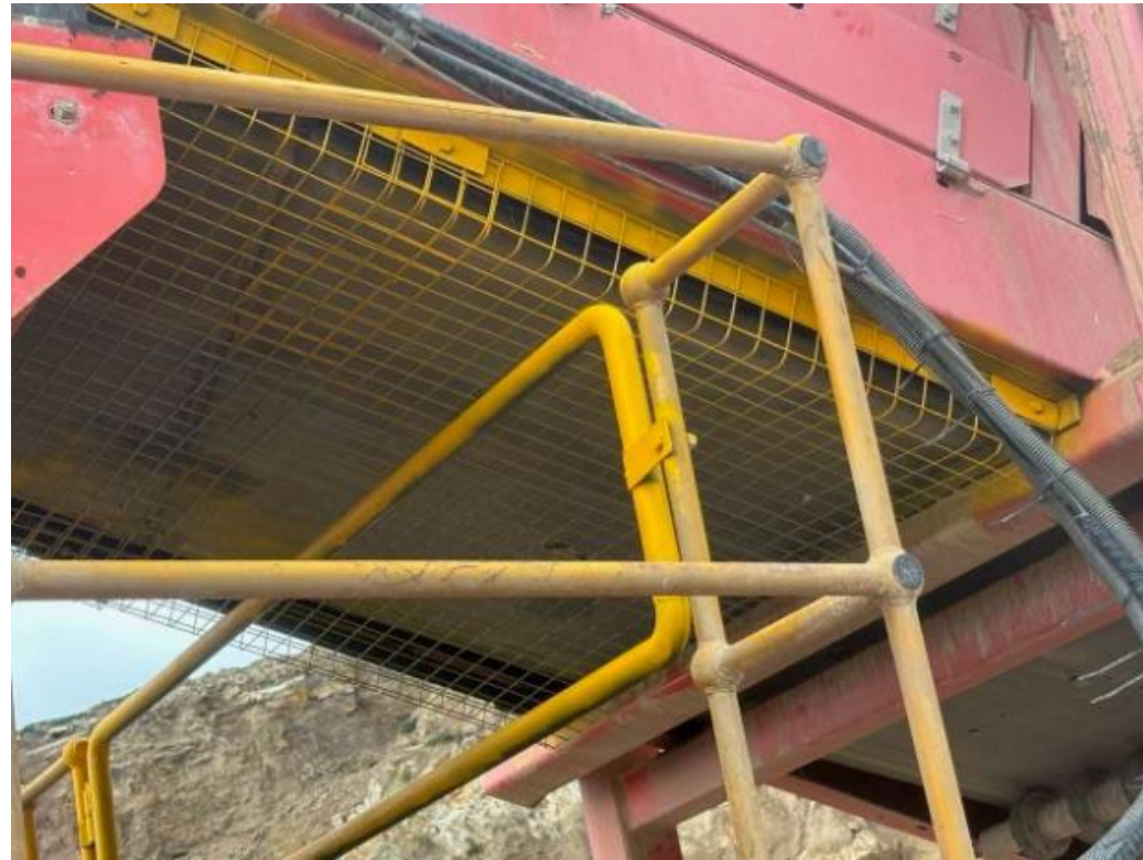
Removable handrail fitted & guarding fitted to underside of belt
