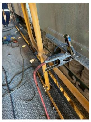
Mine operators should verify that workers carrying out welding activities have identified appropriate earthing points, their personal protection equipment (PPE) is dry, and they are appropriately trained. Welding machines must be isolated when not in use.
