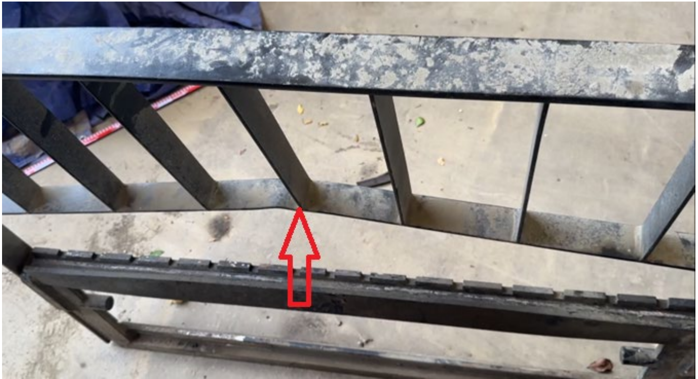
Figure 2: Previous damage to forklift's load guard
