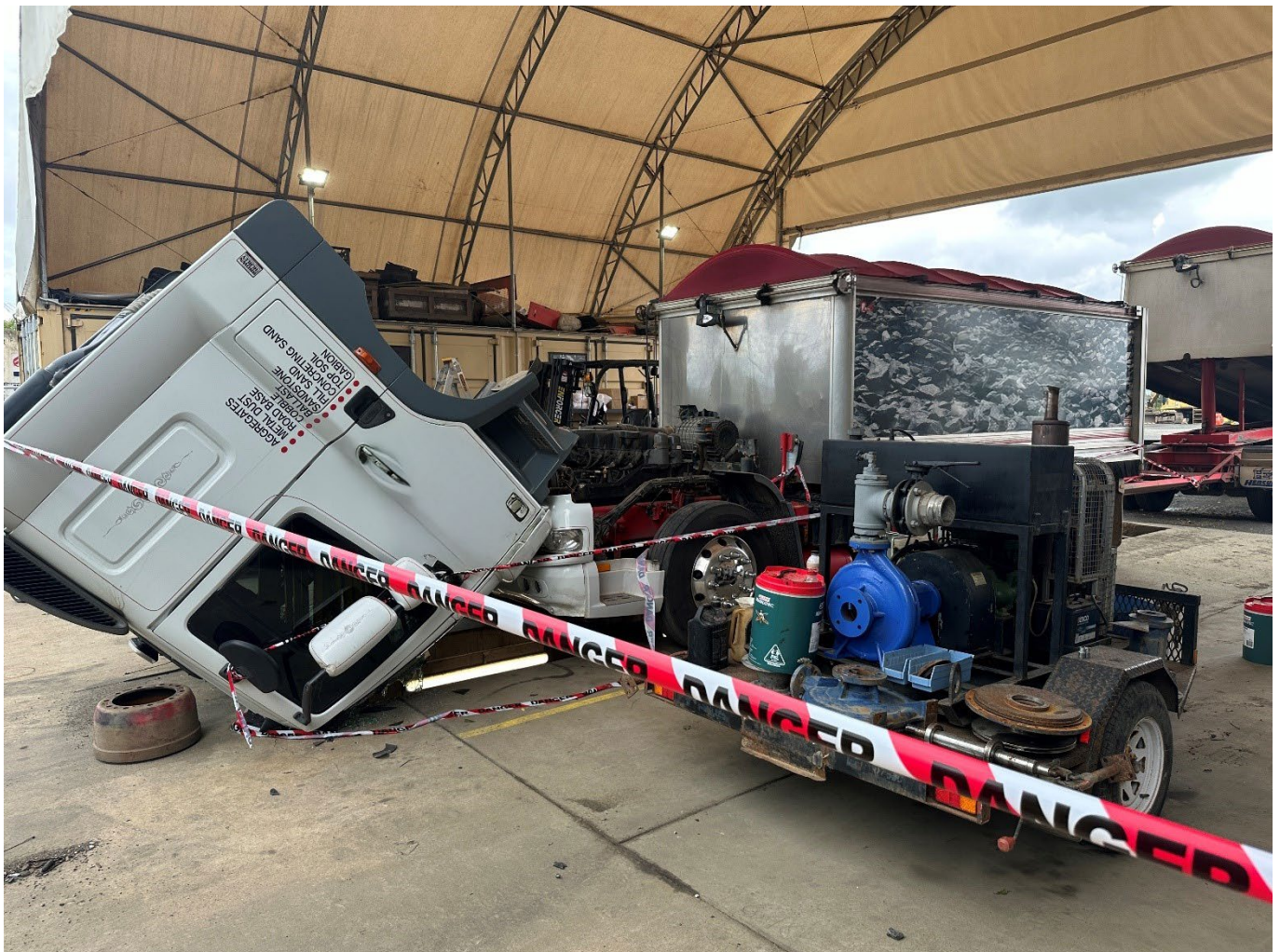
Figure 1: Truck cabin in contact with the workshop ground
