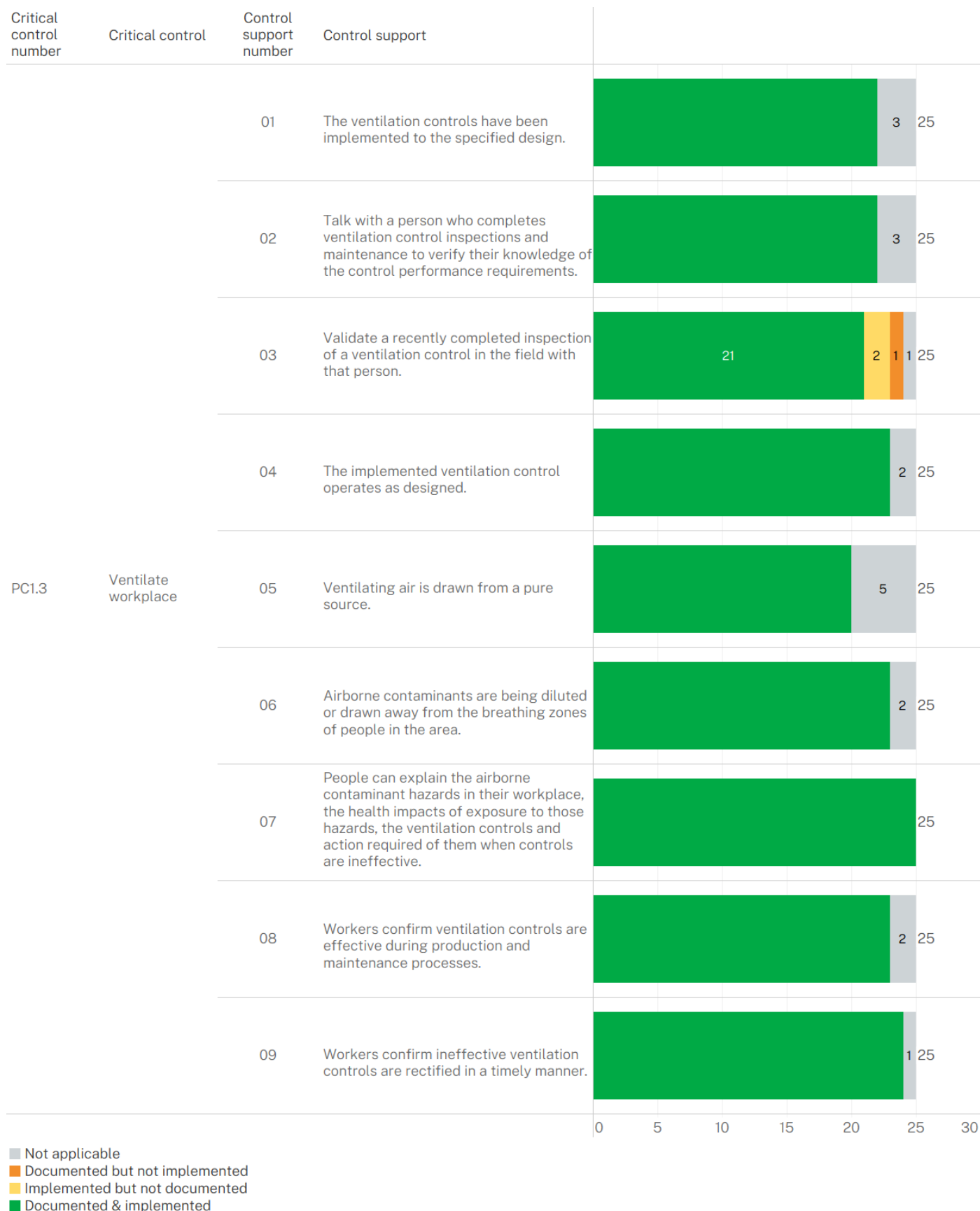
Figure 4: Overall assessment findings ratings by critical control and control support for surface coal mines
