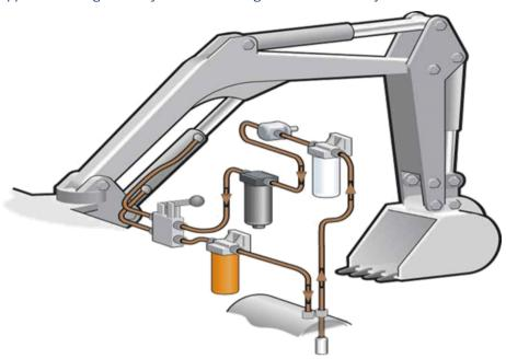
Appendix M - Figure 2 - Hydraulic valve bank with multiple hoses and diffusion sleeves
