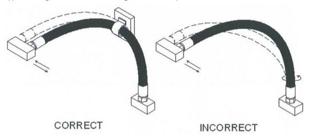
Pressure applied to a twisted hose may shorten the life of the hose or loosen the connections. To avoid twisting, the hose layline or marking can be used as a reference (see Appendix F - Figure 9) if the layline or marking is parallel to the axis of the hose. Twisting can also be avoided by using two wrenches during the installation of swivel connectors.
