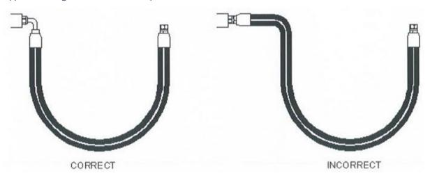
Unnecessarily long hoses can increase pressure drop and affect system performance. When pressurised, hoses that are too short may pull loose from their fittings, or stress the hose fitting connections, causing premature metallic or seal failures. Appendix F - Figures 4, 5 and 6 provide guidance for selecting hose length.
