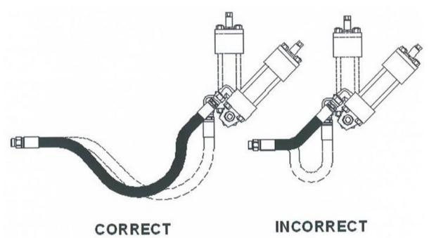
Appendix F - Figure 5 - Hose and machine tolerances
