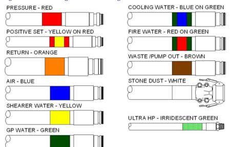
Longwall hose assemblies and/or pipes should have a unique coupling style or size to prevent cross-connection of different circuits.
