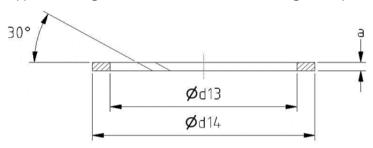
Appendix L - Table 6 - O-ring back-up washer (all dimensions in millimetres)
