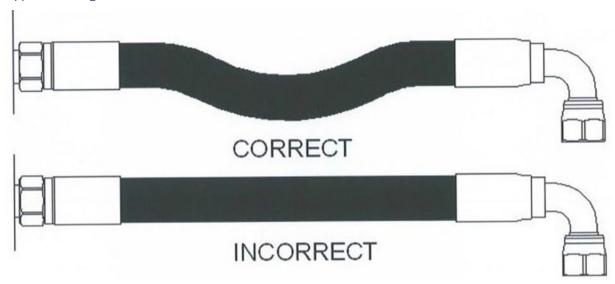
Design hoses to accommodate length changes from changing pressures. Do not cross or clamp together high- and low-pressure hoses. The difference in length changes could wear the hose covers.
