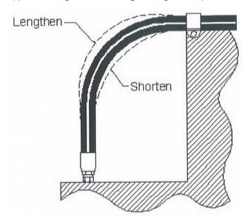
Where hoses are connected between system components that move relative to each other, hoses should be designed taking this into consideration. Avoid multiple planes of motion and twisting motion. Consider the motion of the hose when selecting the hose and predicting service life. In applications that require the hose to move or bend, see Appendix F - Figures 7A, 7B and 8.
